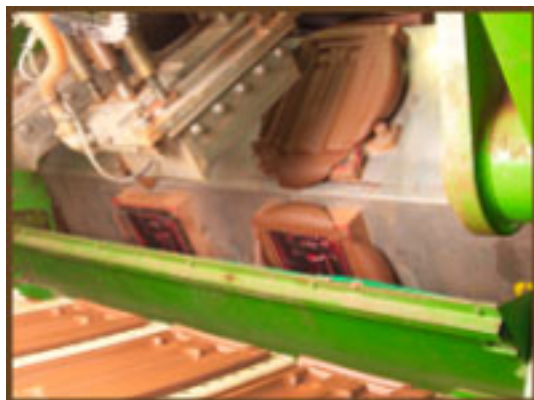
The Press Clay bats are pressed to specific profile molds.
