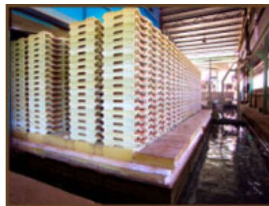
The Kiln Dried tiles are assembled in individual refractory H-supports to be fired at 1,060°C in the patented Hydrocasing Tunnel Kiln for high durability and excellent insulation properties.
