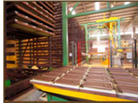
The Drier Pressed tiles are fed to the Drier to eliminate all moisture content.
