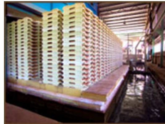
The Kiln Dried tiles are assembled in individual refractory H-supports to be fired at 1,060°C in the patented Hydrocasing Tunnel Kiln for high durability and excellent insulation properties.
